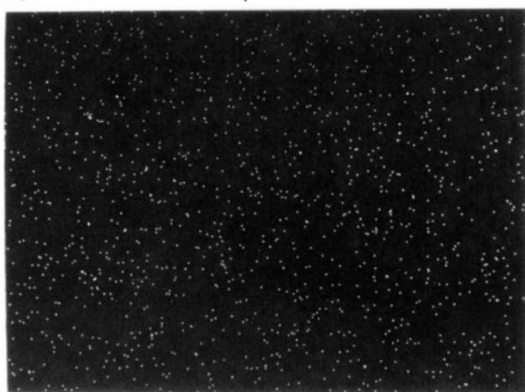
Figure 4. X-ray dot maps of PMDA-ODA/SiO 2 (6%) and PMDA-ODA/SiO 2 (42%). The dots represent concentrations of Si atoms.
